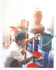
Pot filters for removing arsenic from water
